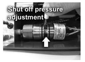
screw driver up to increase pressure; down (counterclockwise) to decrease pressure. Return the plastic collar over the opening before starting.
