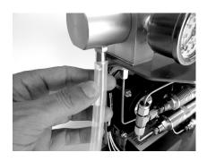
Once you have installed the extraction chamber, slide the silicone hose on the end as shown in picture.
