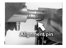
Attach the high pressure hose to the fitting on the end cap. Make sure the locking ring is seated all the way before use. Screw the knob on top of the extractor body clockwise until snug to seal up the vent.
