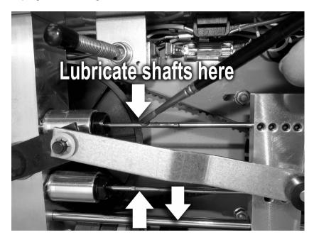
To lubricate both air pistons use **the oil you intend to extract for lubrication or equivalent vegetable oil**. Disassembly of the pistons is not required. Simply put a dab of oil on the exposed piston shafts as shown in the picture using a brush or swab. Once the unit is turned on, the oil will get pulled into the cylinder as the piston moves in and out. See our website videos on the Support page at OCOlabs.com
